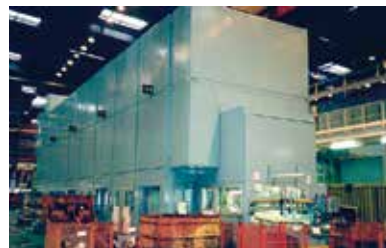
Noise-insulating enclosure, corrugated cardboard machine, SCA, Värnamo, Sweden.
